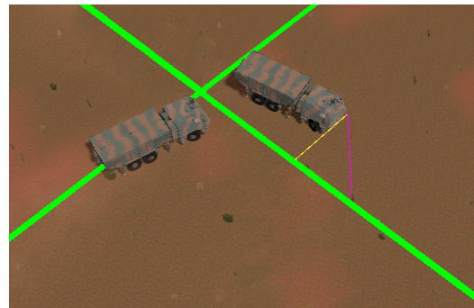
Figure 8. This image illustrate a stopped (waiting) vehicle while the other is following its path. The green lines are the rough path. The yellow line is the vehicle's projected position over the itinerary and the magenta line represents the target position over the itinerary.
