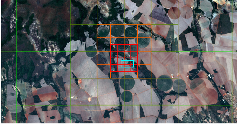
Figure 1: 8 GigaPixel satellite imagery texture rendered at real-time. Each clip region level and its tiles set are represented with colored squares. The cyan rectangle represents the field of view (FOV).
