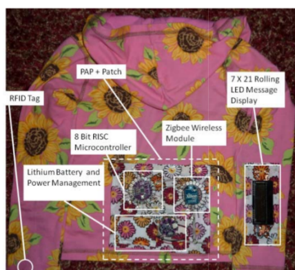
Figure 2: Hoodie used by kids and its components. [Arroyo et al. 2011]
