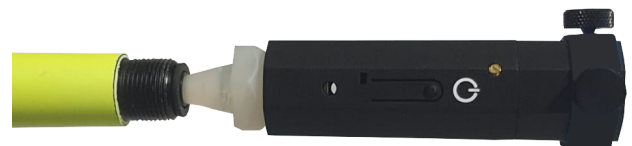
Fig. 7: Laser emitter attached to gun barrel.
