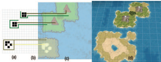
Figure 1. A graphical representation of the method proposed. The patterns in a cellular automaton (a) are translated through a set of rules (b) into generative data structures, here depicted graphically (c) containing information for a rendering process to generate an environment (d).
