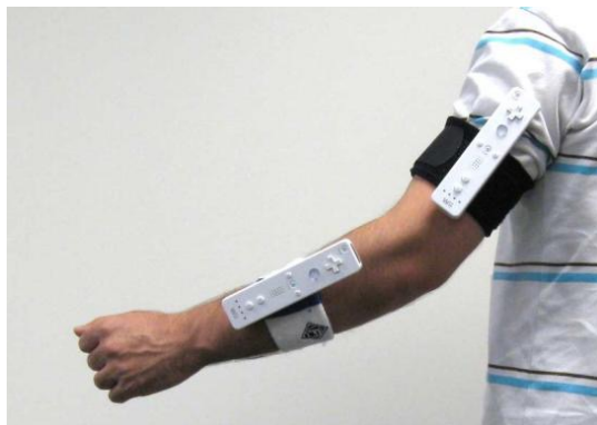
Figure 6: Wiimotes attached by armbands in the arm and forearm [6].
