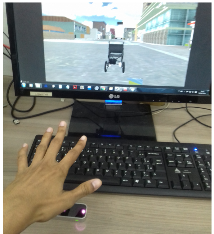
Figure 12: Example of a user controlling a wheelchair through hand gestures.
