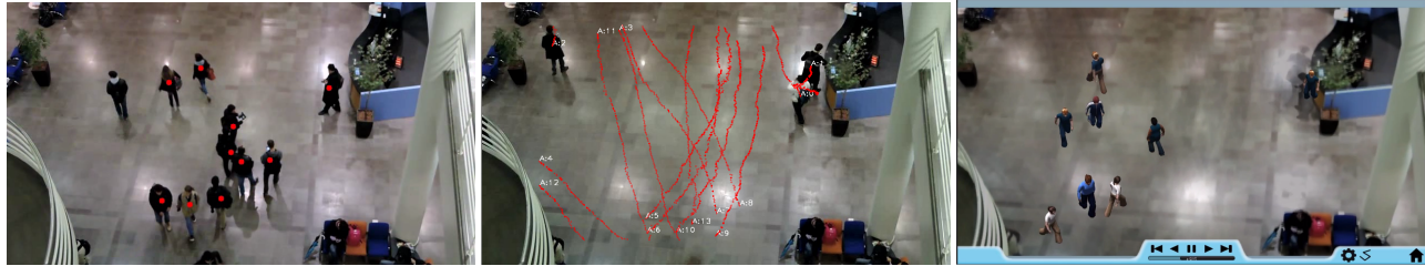
Figure 1: Overview of our method: on the left side real people trajectories are detected and tracked in a video sequence; in the center the trajectories are used to learn patterns of motion in our method, and on the right side our viewer illustrates population for a game, based on real life trajectories.
