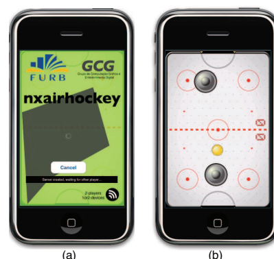
Figure 7: (a) Game connection screen (loaded from a NIB file); (b) NXAirHockey game screen (rendered into an OpenGL canvas)
